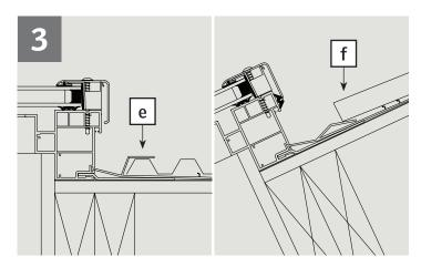
Install roofing around the unit sides under the water diverter gasket (**e**), and over the water diverter gasket at the top (**f**).
