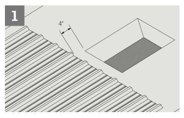
Install roofing to 4" from the bottom edge of the skylight rough opening. Grind or file any sharp edges on the roof panel that are less than 8" from the opening.
