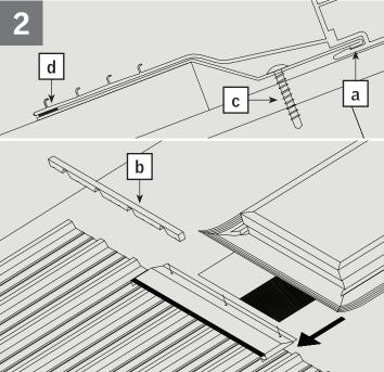
Insert roof adapter into groove under the flange on the bottom edge of the skylight (a). Place skylight over the rough opening.
