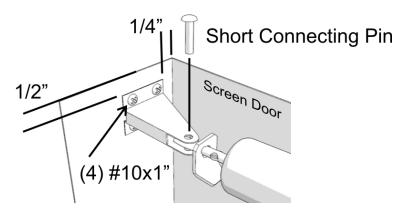
B: Pull closure tube shaft out enough to set "Hold Open Washer".
